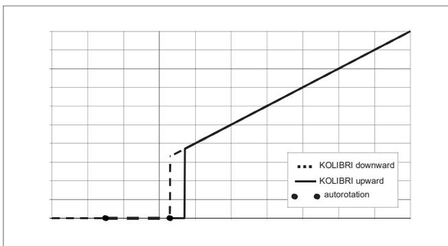
The heli mode operates with real RPM control (governor). The motor RPM speed is kept constant as long as the performance of the battery and motor are sufficient. The ESC stores all parameters of the program, such as the ratio of selected RPM and the head speed at every battery change (performance adjustments are made for each different battery).
