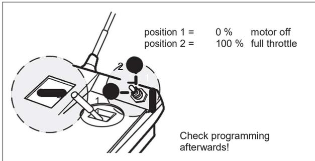
1. Before beginning, set all throttle trims and sub trims to zero, set throttle travel adjust to 100 / 100, and set your beginning throttle curve for programming from 0-100% (see also from 3.1 on).
